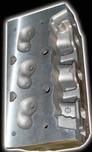
This casting is an NHRA-approved replacement for the GM V-6 Splayed Valve casting, P/N 10134394.
